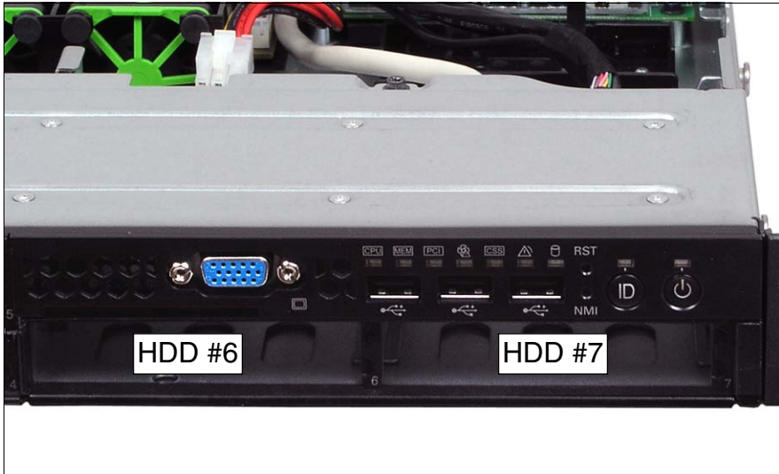
Figure 24: Installation positions of additional HDD modules
